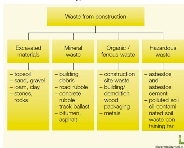
**Figure 1: Composition of waste from construction** Error!
